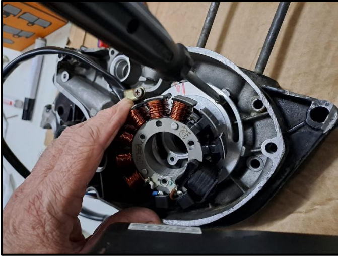
3- Fasten the coil plate and the coil in the shown position.
