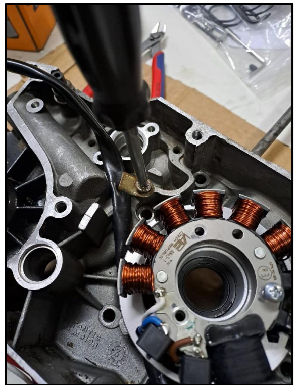
5- Secure the cable in place.
