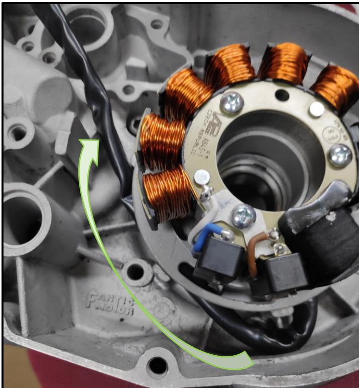
4- Pass the cable through the lower part and bring it upwards.
